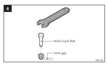
4. Screw in No.8 coach bolt leaving 5mm gap from the surface of the floor.
